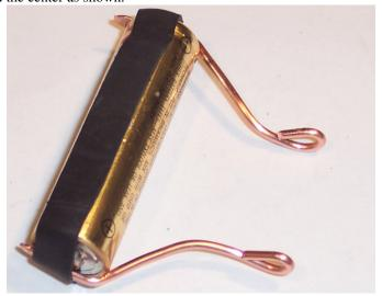
Stick a magnet onto the battery as shown.
