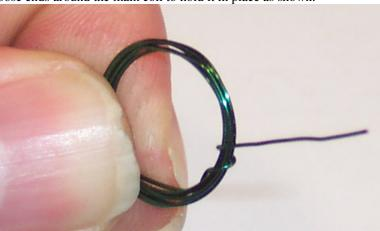
Repeat this wrap for both sides as shown. Do your very best to make sure the coil is balanced. An unbalanced coil may not spin!
