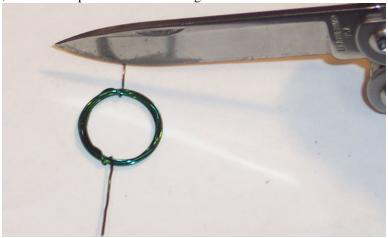
From the **OTHER SIDE**..... Scrape off the insulation from only **ONE SIDE!!!!**
