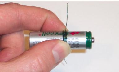
Next wrap one of the loose ends around the main coil to hold it in place as shown.
